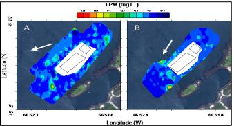
Colour-scaled contour plots of total particulate matter (TPM) (mg L-1) at an aquaculture site based on data collected between 0.5 and 2 m depth on 5 July, 2011 (A) and 6 July, 2011 (B). Arrows indicate the predominant current flow direction during each survey period.
